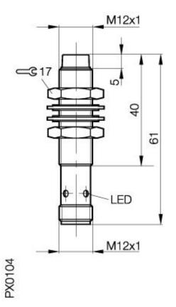
**Inductive Sensors** BES 516-356-S 4-W M12x1 x 61 normally-open Sn=4mm unshielded magnetic field immune
